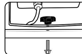
6. Set the floodlights at the ends of the metal support (3) using the metal screws with metal washers(5) with the knob nut type.
