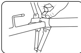
2. Secure the legs by threading the screw.
