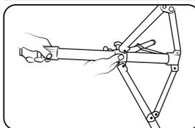
1. Take the metallic tripod base (2), and extend the tripod legs by pushing the central joint to the base.
